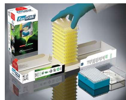
1. Open Fastrak® and grasp transfer top. Lift straight up.
